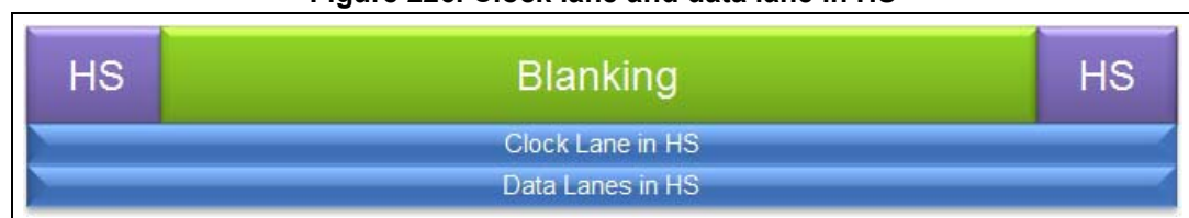
Figure 226. Clock lane and data lane in HS
