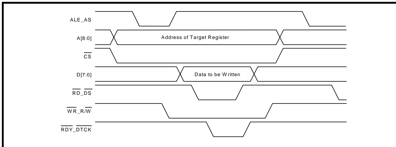
FIGURE 26. MICROPROCESSOR INTERFACE TIMING - MOTOROLA-TYPE PROGRAMMED I/O WRITE OPERATION
