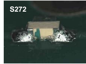
Pin-pad soldering good
