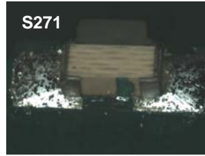
Pin-pad soldering good
