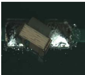
Pin-pad soldering bad
