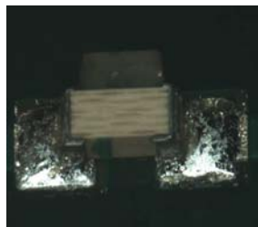
Pin-pad soldering good
