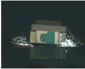
Pin-pad soldering bad
