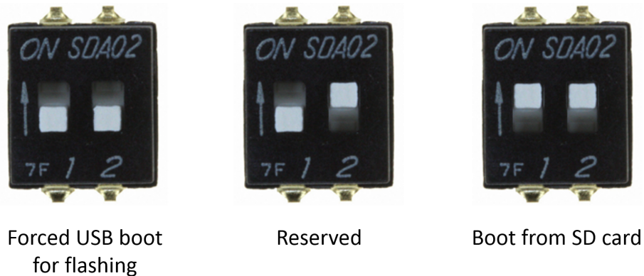
Figure 7. Boot-mode switch SW1
